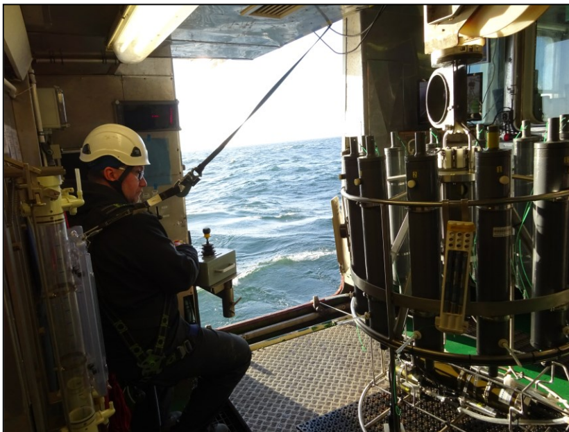
Fig. 4. In the driving seat. Markku Jansson operating our precious Sea-Bird CTD equipped with Rosette bottle sampler, guiding the gear safely through the depths. The occasionally more-or-less inclined horizon did not pose any problems for this crew.
